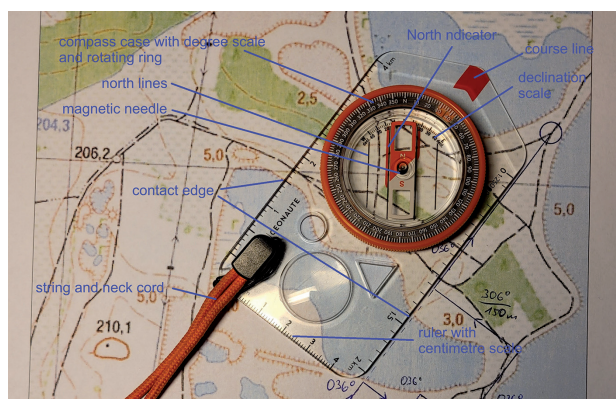
Fig. 7. Construction of a compass.
